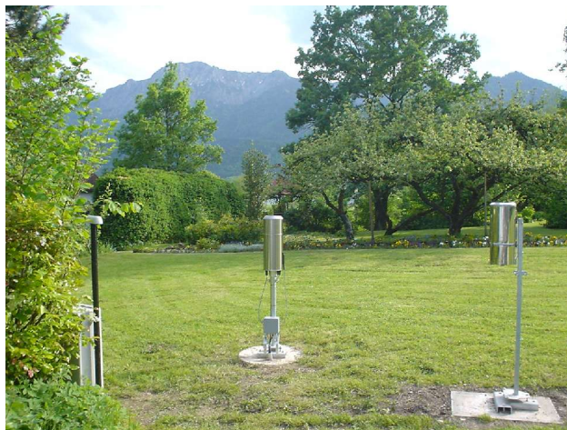
Figure 2. Components of a new precipitation measuring station: computer cabinet with ISDN-data line-access, high resolution pluviometer, Hellmann Gauge (from left to right, not shown: input terminal for additional observed parameters).
