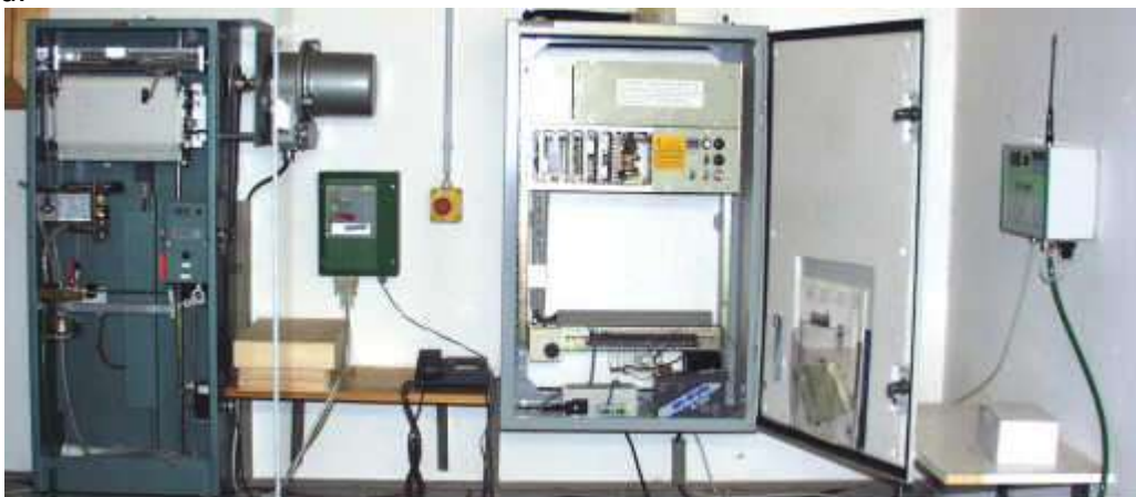
Figure 3. Water Level Gauging Station Freising/Isar (Redundant equipment relative to water level sensors and data logging)
