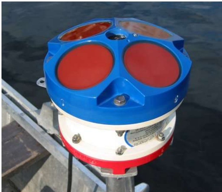
Figure 1. The ADCP Workhorse Rio Grande 600 kHz ADCP of the RD Instruments, mounting position.
