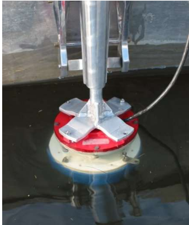
Figure 2. The ADCP Workhorse Rio Grande 600 kHz ADCP in measuring position.
