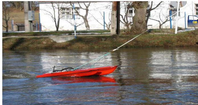
Fig. 2 measurement with trimaran and attached ADCP
