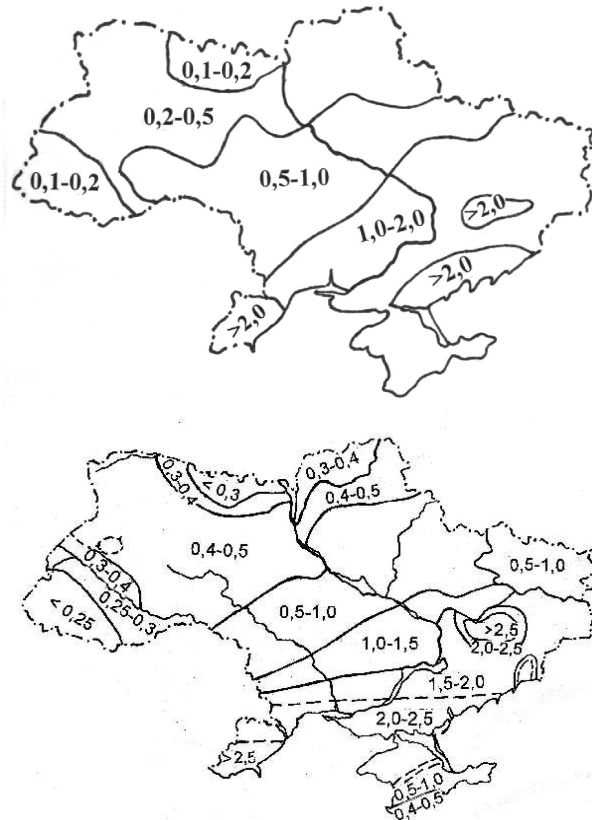
Figure 2. The maps of mineralization of water in Ukrainian's rivers (in g/l): above – in 1947 (the period of low water []), down – nowadays (average data)
