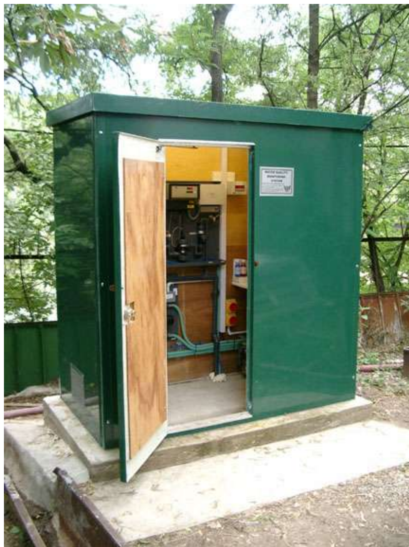
Fig. 3. Automatic control station of water quality on the transboundary rivers Prut and Nistru
